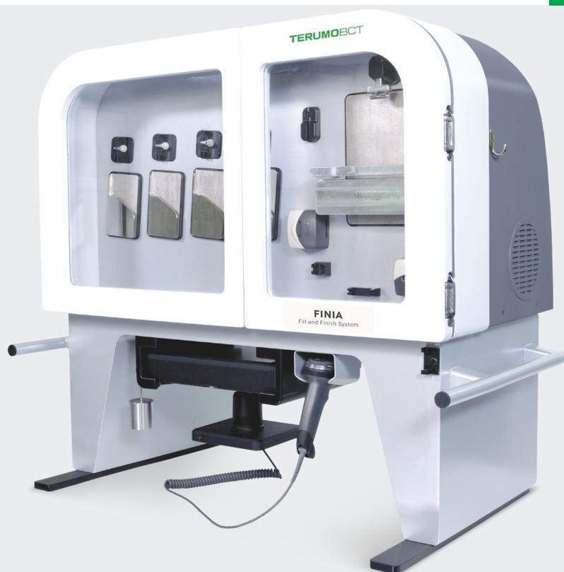
You no longer have to rely on a manual method for your fill and finish step. The functionally closed, single-use Finia disposable tubing sets are designed for use with diverse cell types.
